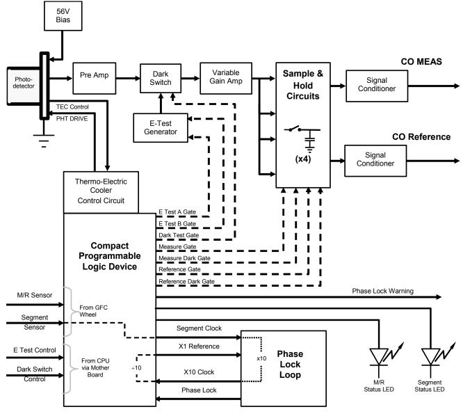
Figure 13-13: GFC7001T/GFC7001TM Sync/Demod Block Diagram
